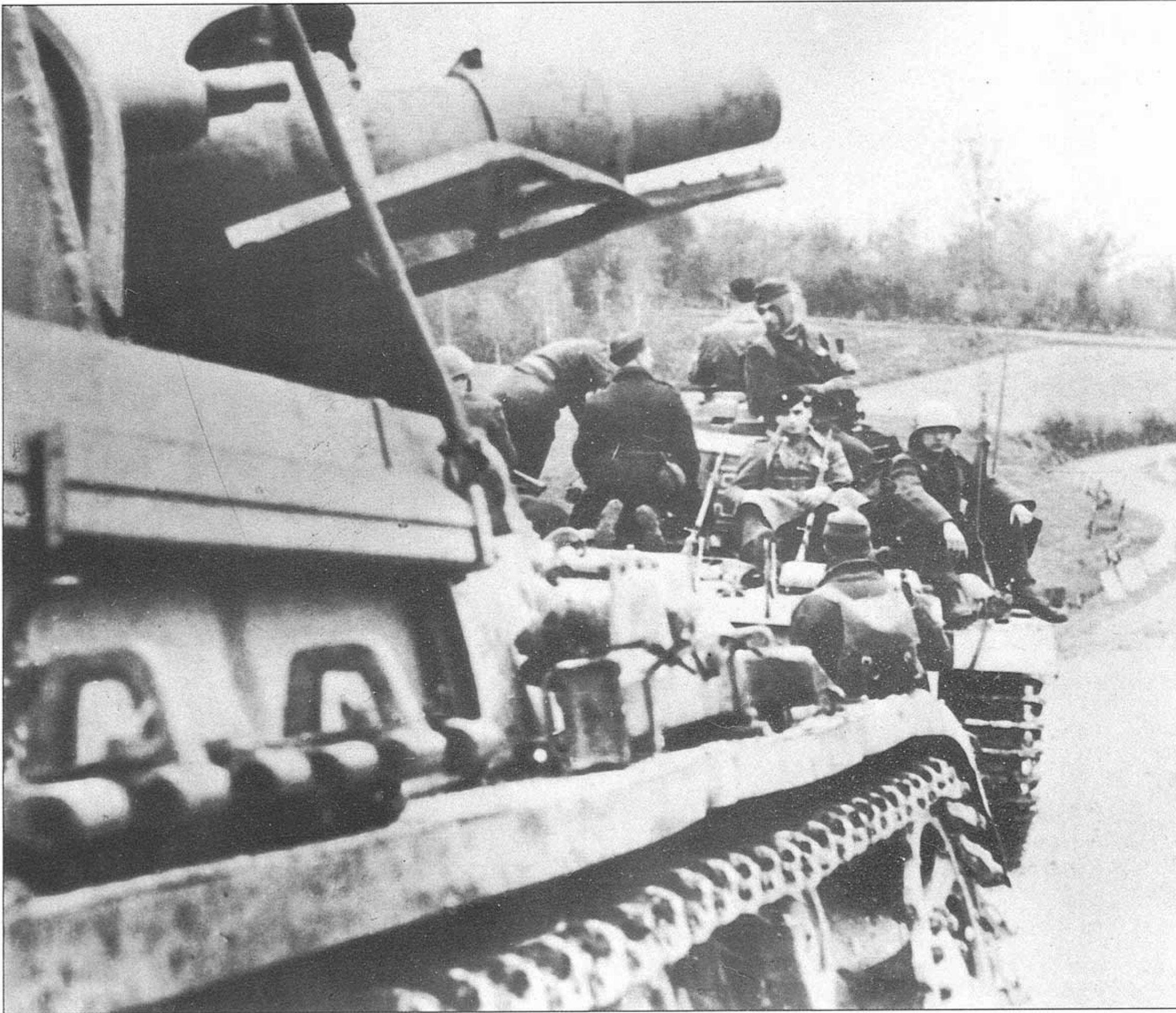
Above: Infantry ride into combat aboard Pz Kpfw IV Ausf E tanks, equipped with short-barrelled 75mm main armament. The metal frame under the barrel of the tank in the foreground is an antenna deflector, designed to bend the radio aerial out of the way of the gun barrel when the turret was traversed.
