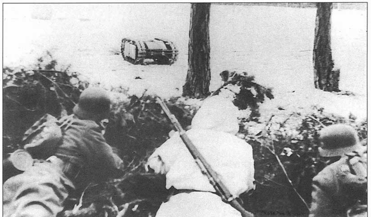
Right: German engineers send a remotely controlled tracked vehicle, known as a Goliath, towards an unseen obstacle. The Goliath, usually driven by an electric motor, contained a 183lb (83kg) explosive charge in the front compartment and a 6562ft (2000m) cable-drum in the rear. Once in position, it was detonated, clearing a path.
