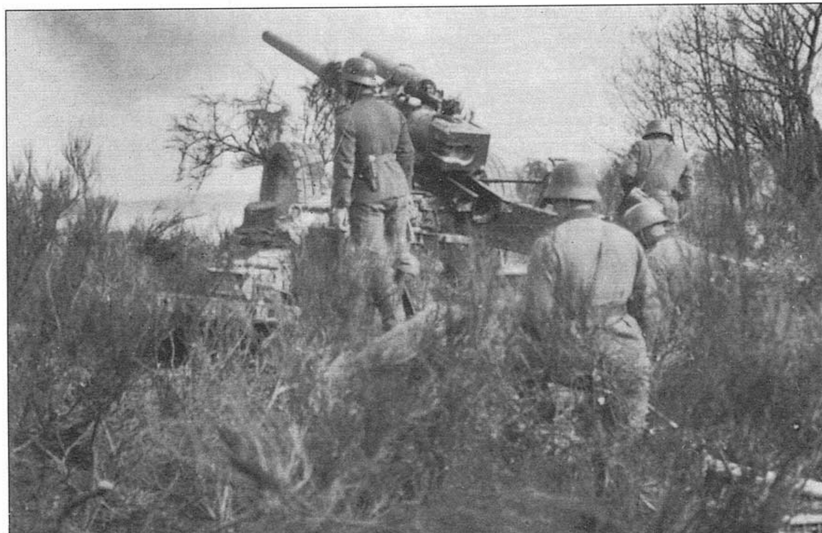
Right: German gunners fire a schwere Kanone 18 in action, 1939. Developed between 1926 and 1929 by Krupp and Rheinmetall, the 100mm K 18 was accepted for issue to artillery units in 1933-34. It remained in production until 1943, having seen widespread active duty throughout the early blitzkrieg campaigns. It was a powerful weapon.
