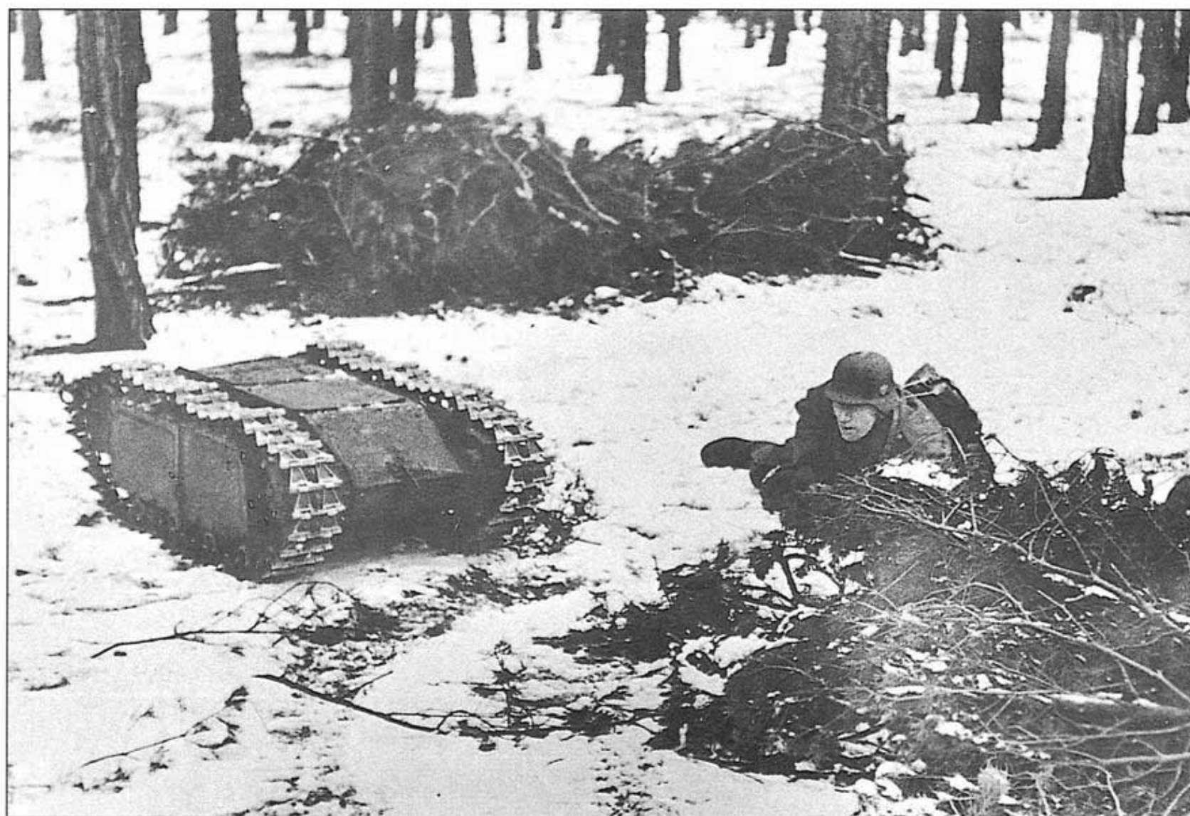
Right: A Goliath remotely controlled demolition device is prepared for action, 1943. The Goliath was often used to attack enemy tanks as well as to clear obstacles: if the device could be positioned beneath the tank and then detonated, it could have a dramatically destructive effect.
