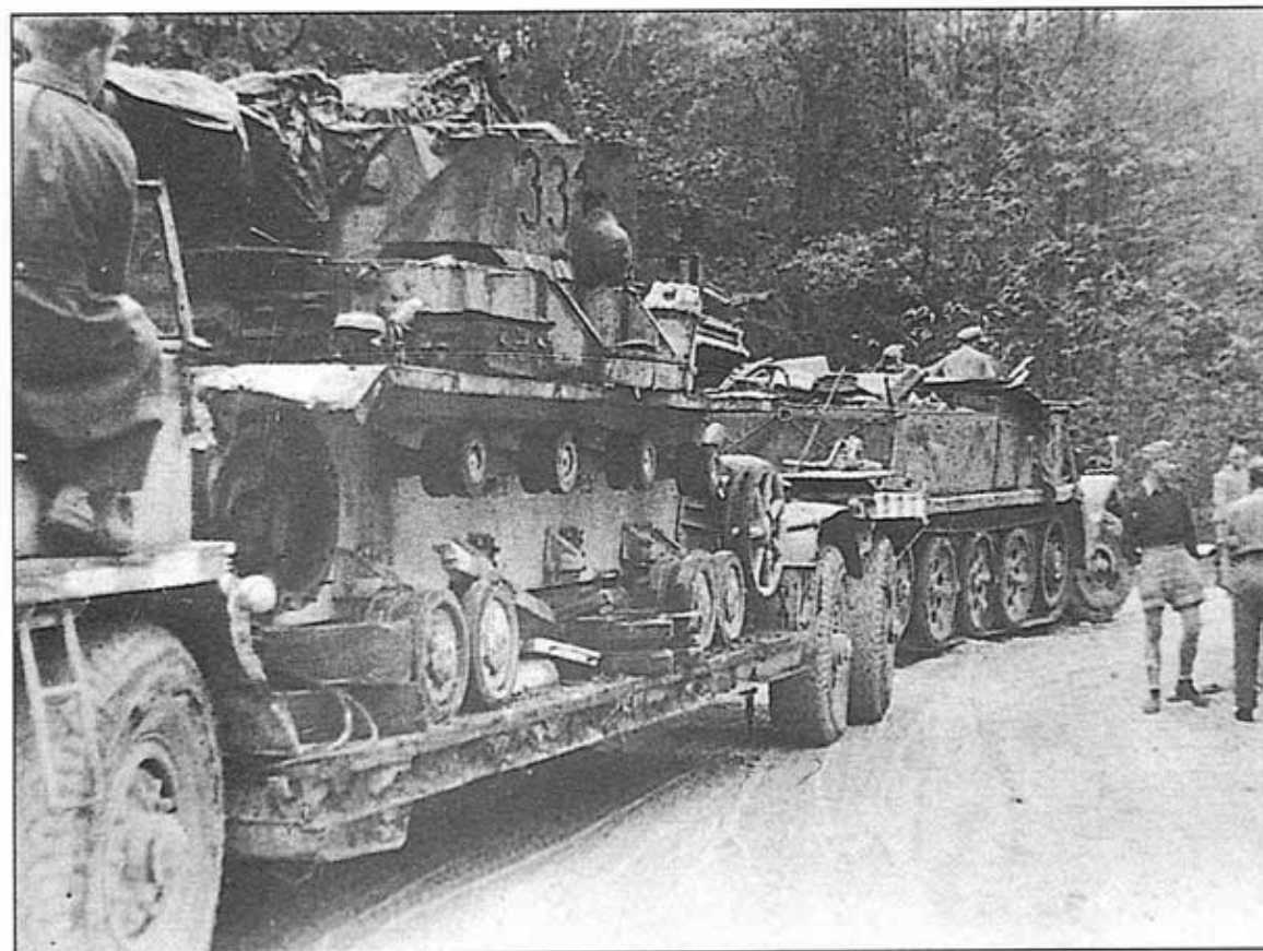
Below: A schwere Zugkraftwagen (sZg Kfz) 18 heavy artillery tractor is used as a recovery vehicle on the narrow roads of central Yugoslavia, April 1941. The trailer it is towing carries the remains of a Pz Kpfw IV Ausf G, damaged by what would appear to be an anti-tank mine which has destroyed a track.
