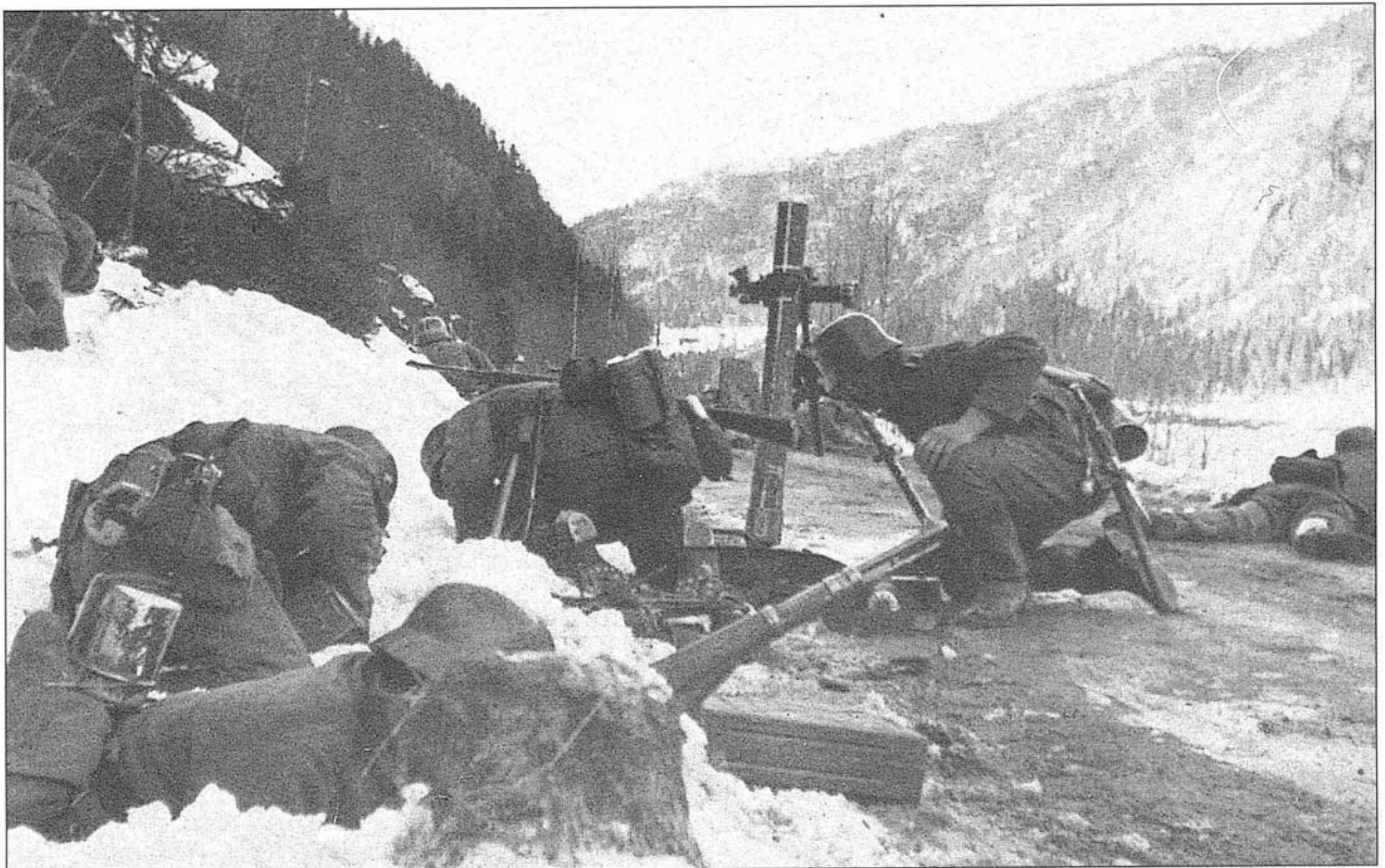
Above: Mountain troops in Norway fire their 80mm Granatwerfer 34 mortar towards enemy positions. The terrain is rugged and the weather cold; one of the results is that the mortar has been positioned with its base-plate on the roadway - not the ideal way to absorb the shock of firing.
