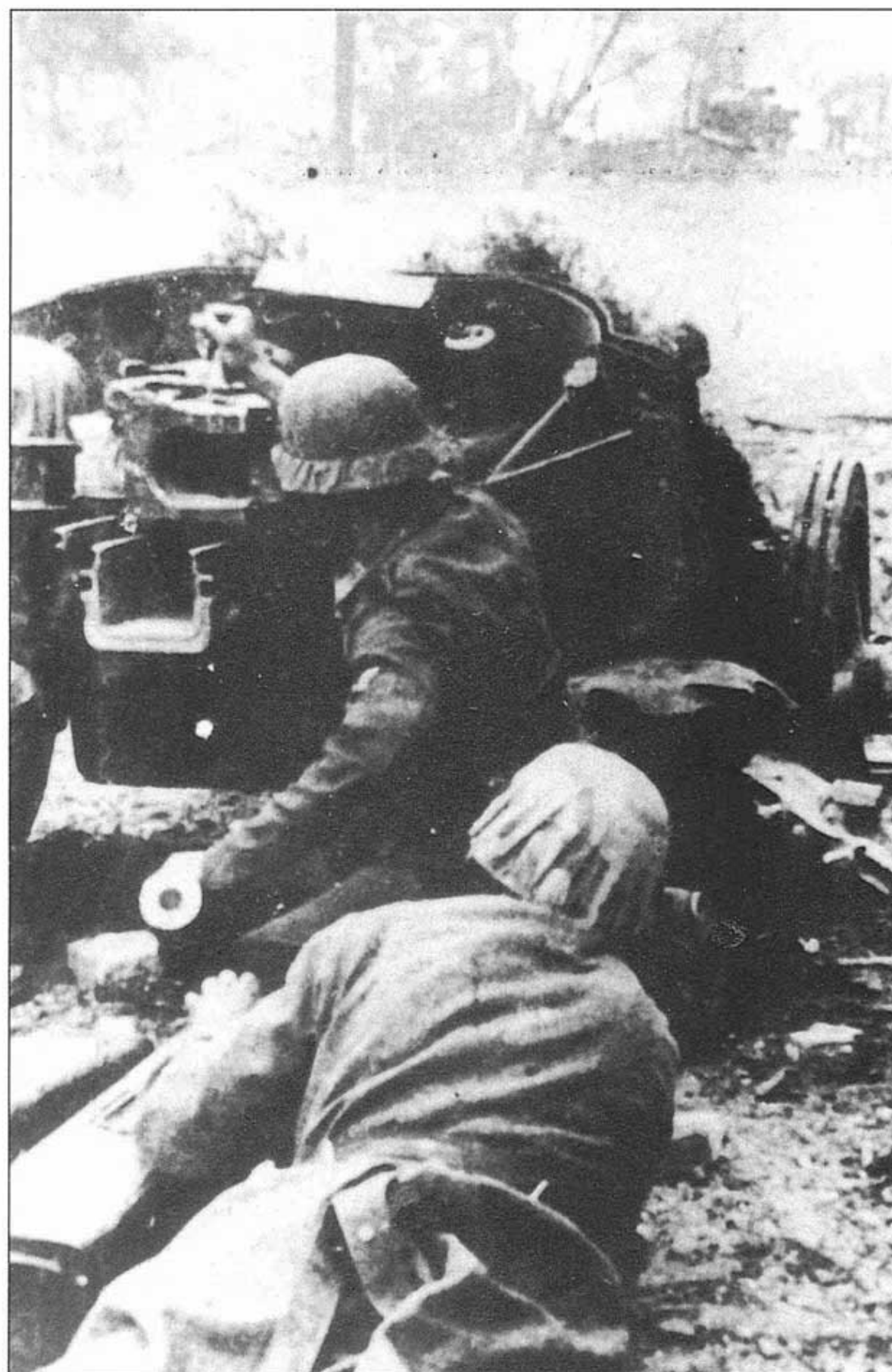
Above: The crew of a 50mm Panzerabwehrkanone (Pak) 38 anti-tank gun in action at the Battle of Kursk, July 1943. Introduced in 1941 as a replacement to the 37mm Pak 35/36, the Pak 38 was a well designed and effective weapon. Its tungsten-core AP40 shells could penetrate almost all types of Allied and Soviet armour:
